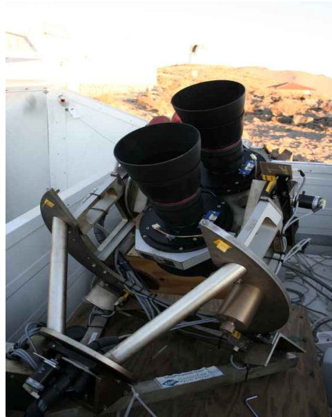
Fig 3. Prototype in LCO after upgrade in June 2006 with CANON EF objectives f=85\text{mm}
